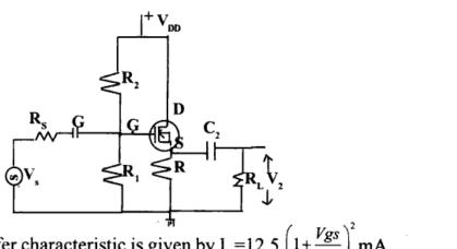
The transfer characteristic is given by  $I_D = 12.5 \left(1 + \frac{Vgs}{2}\right)^2 \text{mA}$  (8)
