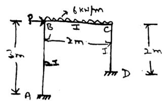
Using slope - deflection method calculate Bending moment and draw Bending moment diagram and deflected shape of the frame.
